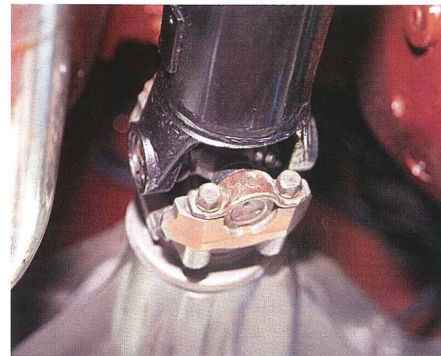
These white inspection marks are on the rear U-joint straps.
