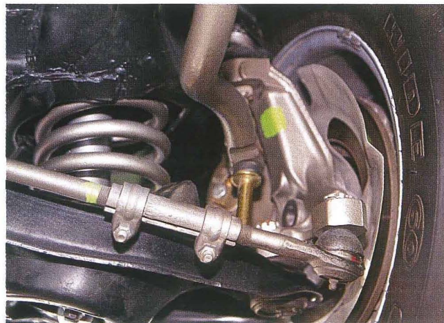
On the driver-side spindle there is a green mark near the top ball joint and another green mark near the tie-rod adjustment.
