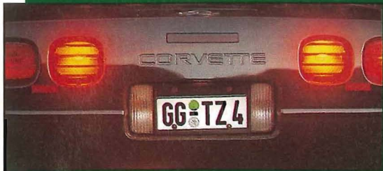
Red rear fog lamp (mandatory in many European countries), rear reflectors, and blanked-out center brake lamp (illegal in Europe).
