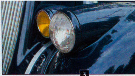
3. Herbert M. Dawley designed and patented the famous fender-mounted headlamps in 1913. The final version of these lights, found on the 1936-38 models, were very bullet-like. The foglights inset neatly between the grille and headlamps.
