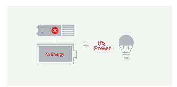
All the energy pulled out of the battery is passed through a single inverter inside the energy storage unit. If this one inverter fails, your battery is essentially useless. That's a lot of responsibility riding on just one piece of the puzzle.
