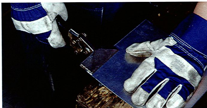
Use a hand seamer to make bends. To bend a safe edge, place \frac{3}{16} inch of metal in the seamer's jaws.
