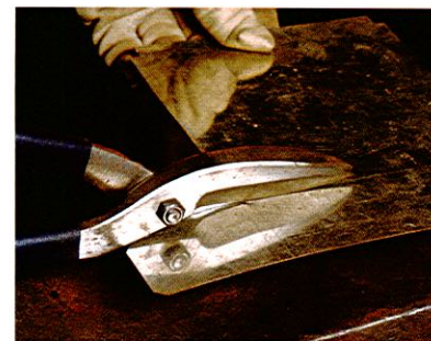
To cut a hole in sheet metal, first use a hollow punch to make a small hole inside the diameter of what will become the large hole. Then insert the tip of the snips into the punched hole. Cut in a circular pattern until the layout line is reached. Follow the layout line to complete the cut.
