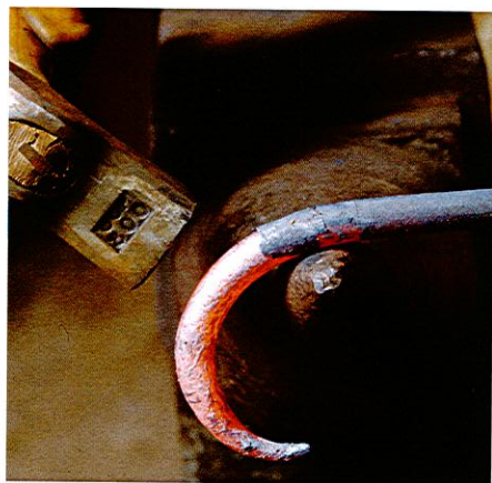
Hot steel can be bent over the horn of an anvil.
