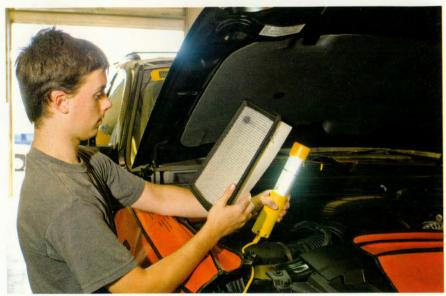
Checking the air filter
