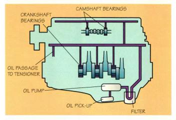
Lubrication system components
