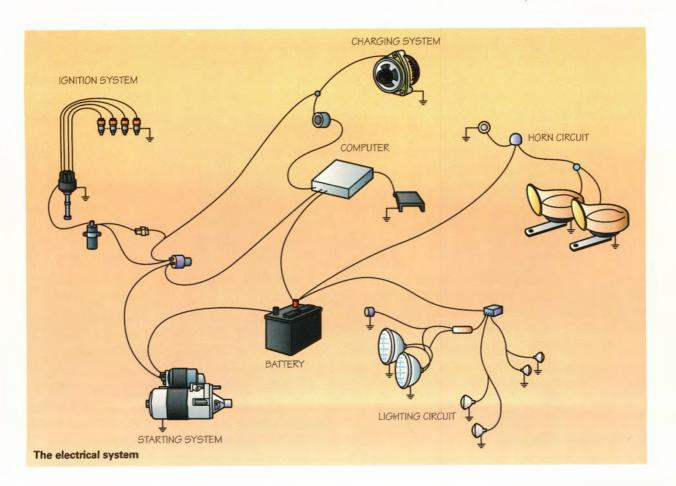
Ignition coils transform 12 volts of electricity into 40,000 to 50,000 volts.
