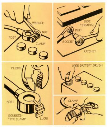
Battery connections must be clean and tight.
