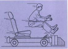
Why are safety belts necessary? Take this example: A man is riding a simple vehicle at any speed, and the vehicle stops suddenly. The rider does not stop until he hits another object. Had a safety belt been in place, the rider would have stopped while still in the seat.
