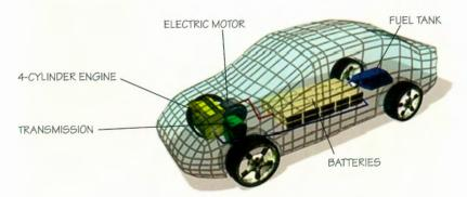
Gasoline-electric parallel hybrid drive train
