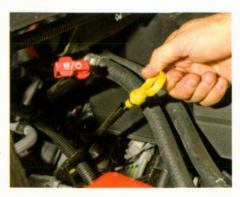
If you change oil yourself, you should dispose of the used oil properly. Put it in a leakproof container, label it, and take it to a recycling facility. Do the same with used oil filters.
