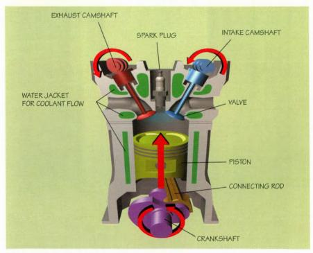
**Combustion chamber components**
