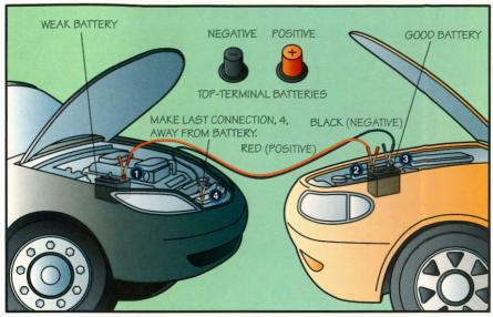
Correct jumper cable connections
