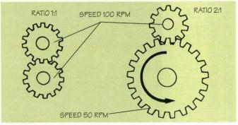
The ratio between the size of two gears affects the torque the gears generate.
