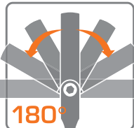
180° flex head has 13 Locking Positions.
