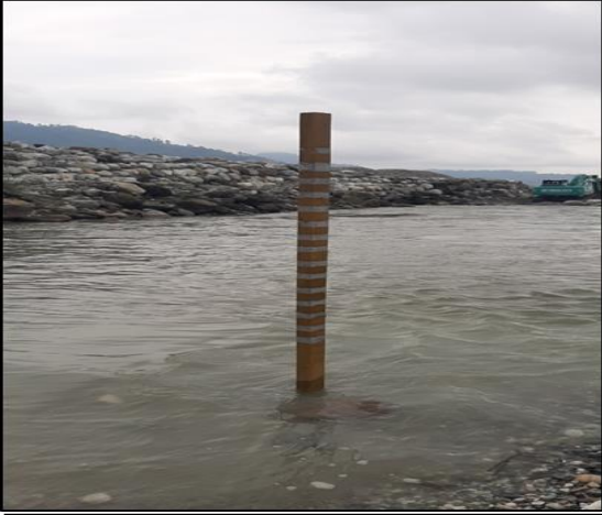
Staff installed at two locations along the Ammochhu to measure change in water level
