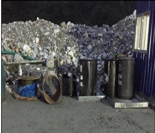
Steel trays used to store open oil barrels
