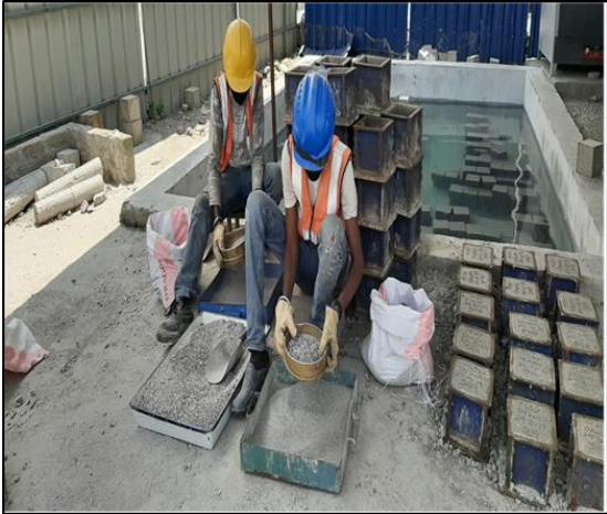
Trays used to segregate sand and aggregates
