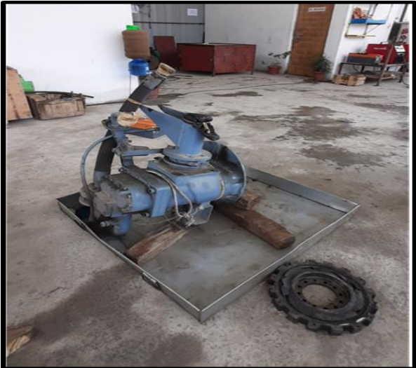
Preventive measures at workshops to avoid ground contamination
