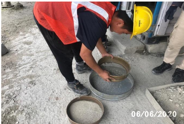
Coarse aggregate gradation test
