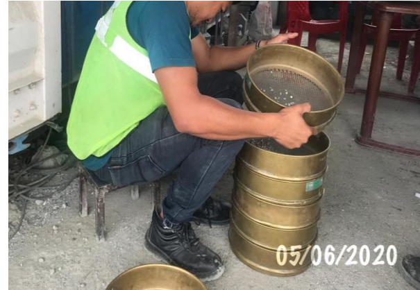
Fine aggregate gradation test
