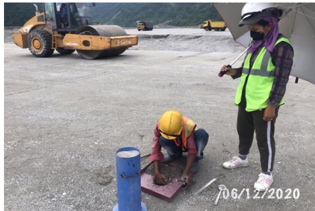
OMC test after compaction
