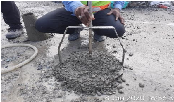
Slump test and concreting for dead man anchor blocks
