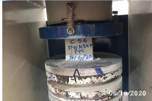
Compressive strength test
