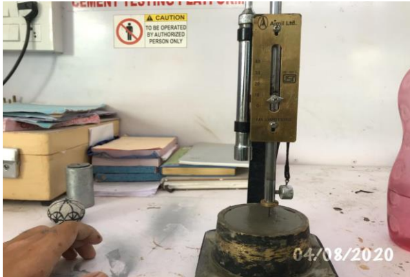
Initial and final setting time for cement
