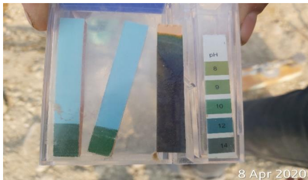
Bentonite pH test
