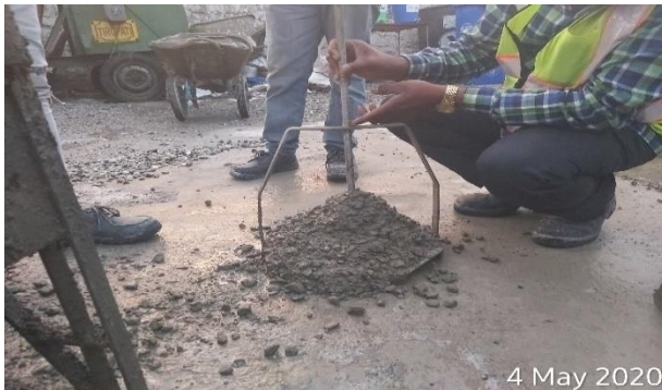
Slump test and concreting for Shear
