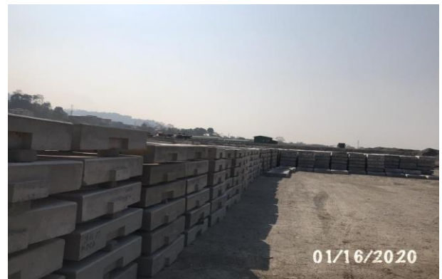
Curing and stacking of grass paver precast blocks
