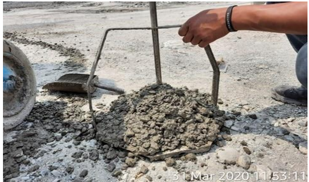
Slump test for Cast in-situ wall
