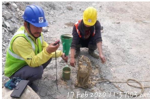
Bentonite viscosity test
