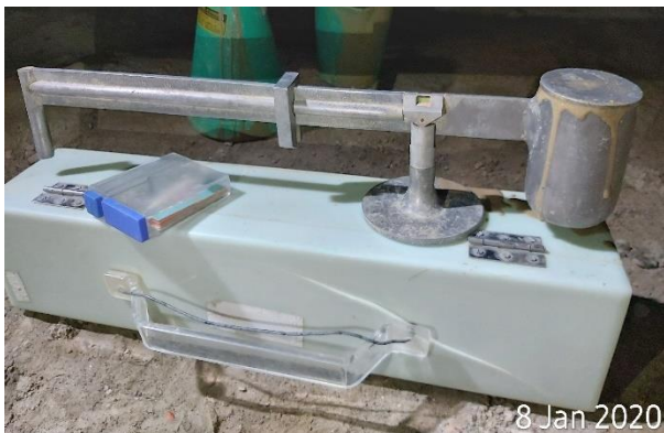
Bentonite density test
