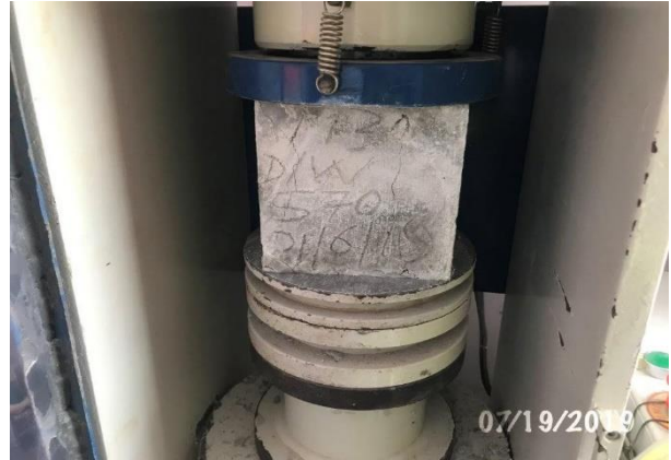
Concrete cube testing
