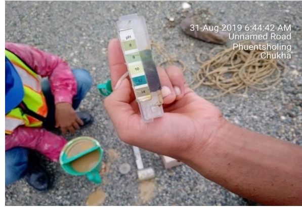
Bentonite pH value test
