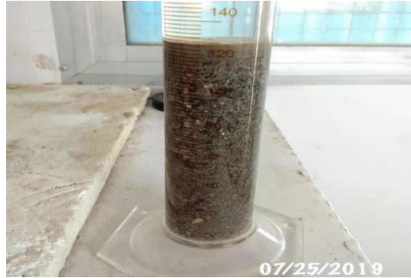
Silt content test
