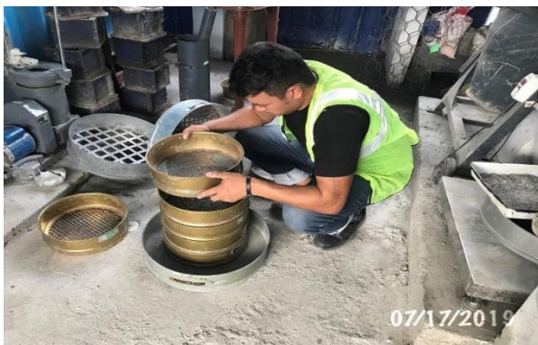
Fine aggregate gradation test
