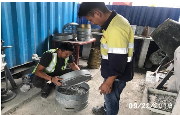
Coarse aggregate gradation test
