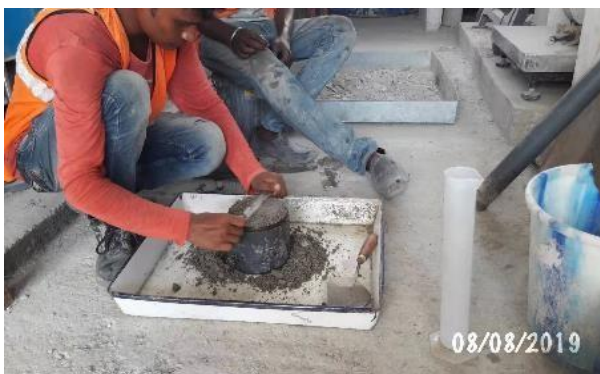
MDD test at site lab
