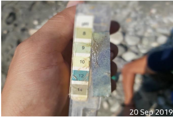
Bentonite pH value test
