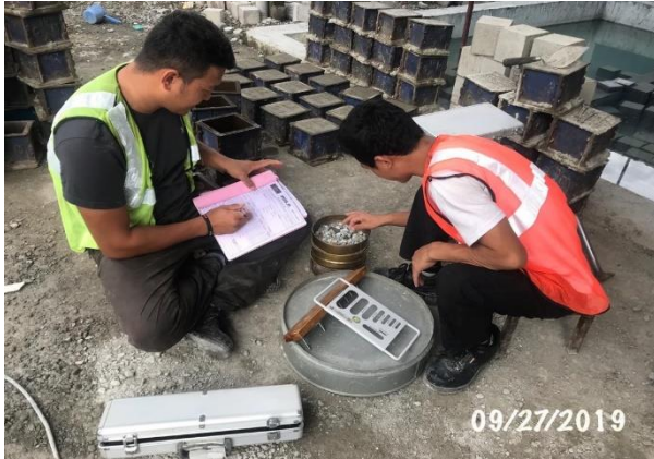
Flakiness and elongation index test
