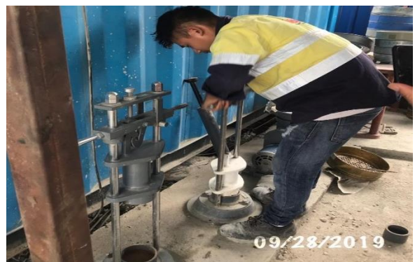
Impact value test for coarse aggregate
