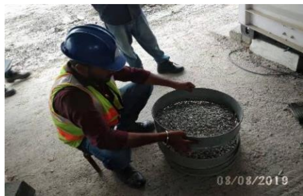
Coarse aggregate gradation test
