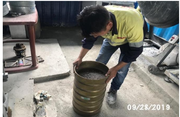
Fine aggregate gradation test
