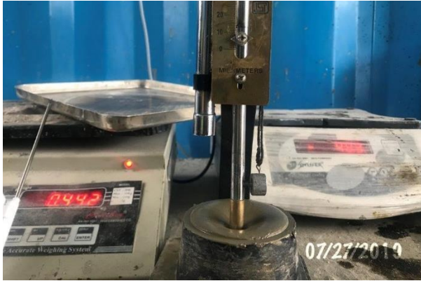
Initial and final setting time for cement
