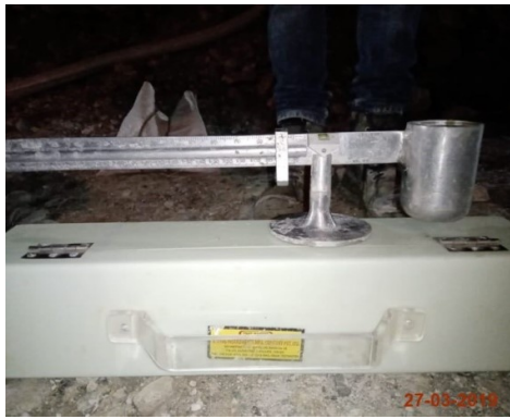
Bentonite density test
