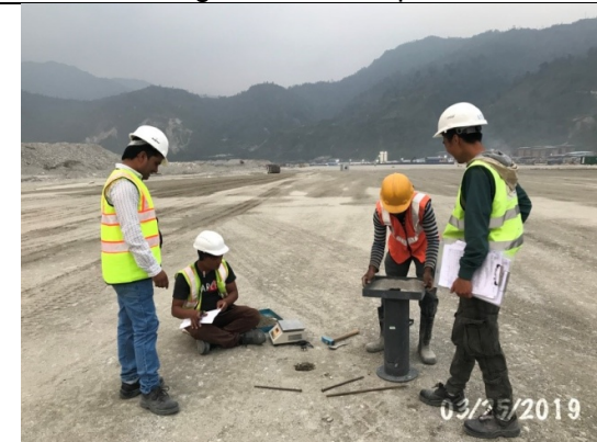
Field density tests
