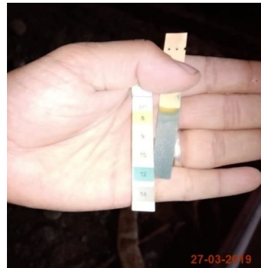
Bentonite PH test
