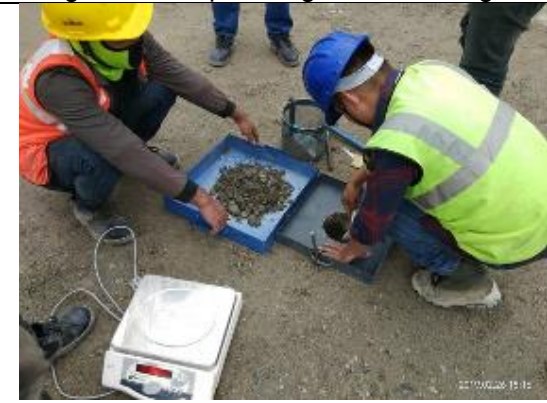
Field density tests
