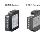
Existing general phase-sequence/phase-loss and other relays use the condenser voltage divider method, which could lead to heating caused by inverter noise. The K8AK/K8DS Series ensures safe and reliable use by employing the switching-mode power supply method, which prevents heating caused by inverter noise and similar factors.
