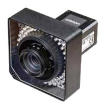
The new V440-F Series offers advanced decode algorithms and improved data output configuration especially for Matrix reading. The V440-F expands on the strength of V430 platform with high resolution sensor and C-mount lens for wider configuration of working distance and Field of View.
