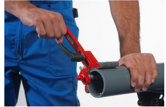
Step 3: Chamfer the pipe
