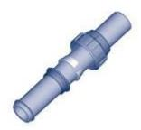
1. Cut the pipe square at 90° to the length using a pipe cutter. Lubricate the pipe and the gasket so that the fittings sit correctly on the pipe. Insert the fittings onto the pipe in the following order: ring nut clinching ring, thrust bushing and put the gasket on the mouth of the pipe.
