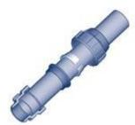
2. Push the body of the fitting on the pipe until the gasket is pushed inside the body (fig.2)
