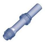
3. Untighten the nut, open the clenching ring and insert it on the pipe, fully tighten the nut using a belt or chain wrench.
