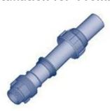
1. Cut the pipe square at 90° to the length using a pipe cutter. Lubricate the pipe and the gasket so that the fittings sit correctly on the pipe. Insert the fittings onto the pipe in the following order: ring nut, clinching ring, thrust bushing, gasket and body of the fitting.
