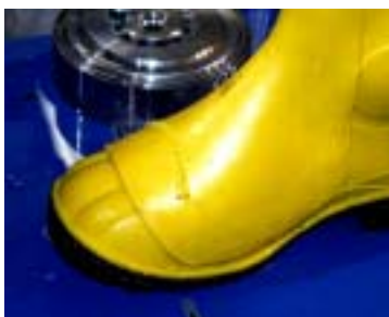
Front part of the boot after stress
